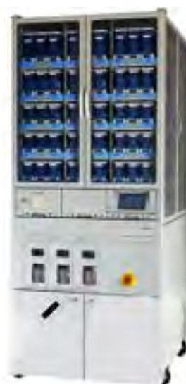
Figure 15: Automate Robotik Technology® AP-405® [35]
