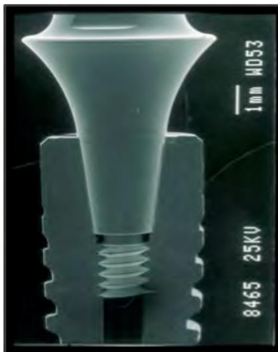
Figure 59: Connection Cône Morse d'un implant Ankylos. Image Ankylos. Dentsply
